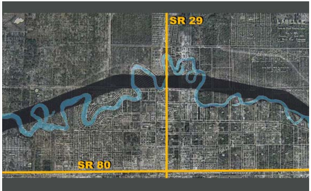
Compare sizes of the old (blue) and new (black) river through LaBelle.
